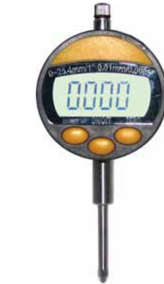
110-F001 数显百分表 digital dial indicator Size:0-25mm 0-1"
