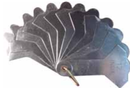
WG-03 焊缝规 Weld seam gauge with 12 blades 12 blades, held fan-form by a ring. (3/3.5/4/4.5/5/5.5/6/6.5/7/8/10/12mm) for checking welding seams in right-angled corners.
