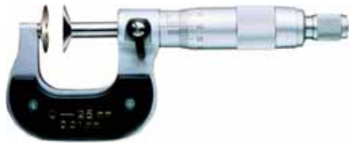
110-B003 碟型量面千分尺 (公法线千分尺) Disk shape head micrometer, be used for measuring gear wheel's base tangent Size: 5-30mm 50-75mm 25-50mm 75-100mm
